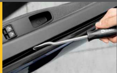
TOOL FOR REMOVING GLASS SEALS
