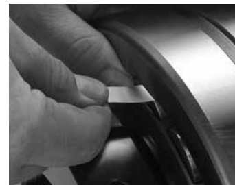
Fig. 97. Measure of RIC before installation.
