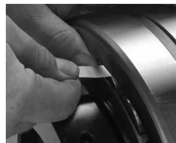
Fig. 95. Measure RIC before installation.
