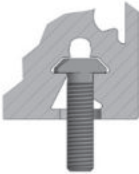
Figure 6.7 ___ Linear Axis AXF with hammer screws
