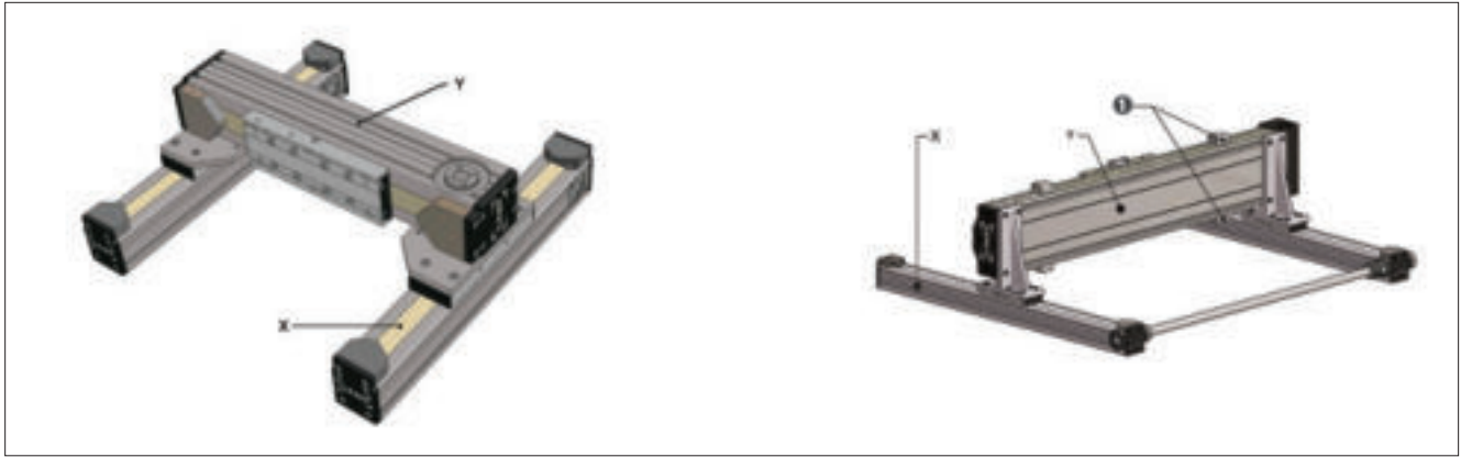
Figure 6.14 __ Gantry connection AXC / AXC and AXC / AXDL
