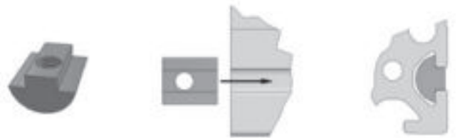
Figure 6.5___ Sliding block designs
