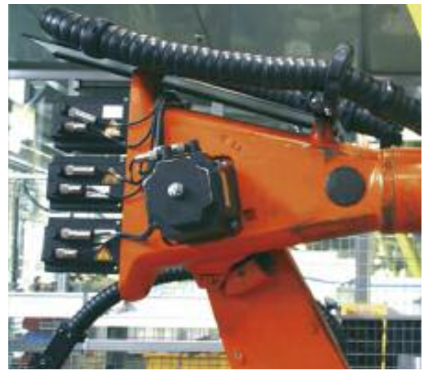
Triflex® RS - Extremely flat design, guides close to the robotic arm
